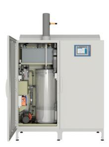
CHLORINSITU IIa is a compact on-site electrolysis system for the production of a low-chlorate hypochlorite solution from sodium chloride and electrical energy. A key advantage is its simple process management and excellent system safety through integrated ventilation and bleeding.
