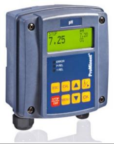
The DULCOMETER<sup>®</sup> Compact controller is a one-channel PID controller for the measured variables pH, ORP, chlorine and inductive conductivity. It can monodirectionally control the measured variable, monitor limit values and transmit the measured value via an mA output, e.g. to a PLC. The mA output can optionally also be configured as a controlled variable output. The controller has one pulse frequency output to control one metering pump. One output relay can optionally
