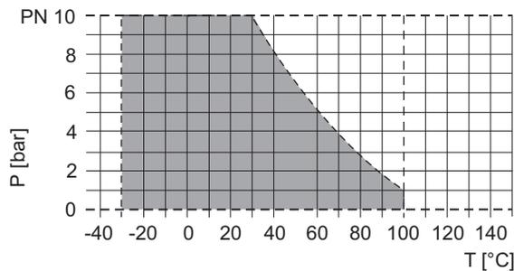
Fig. 10 Pressure and temperature limits PVDF, PTFE, V4A
