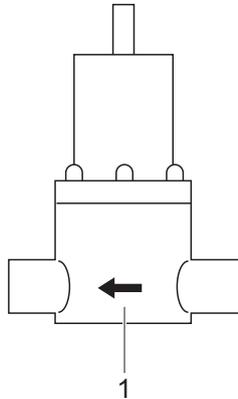
Fig. 3 Fitting with directional arrow (example)
