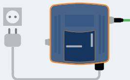
Start the **DULConneX Gateway** by connecting the power cable.
